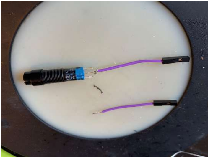
Loop the jumper wire around the button hooks
