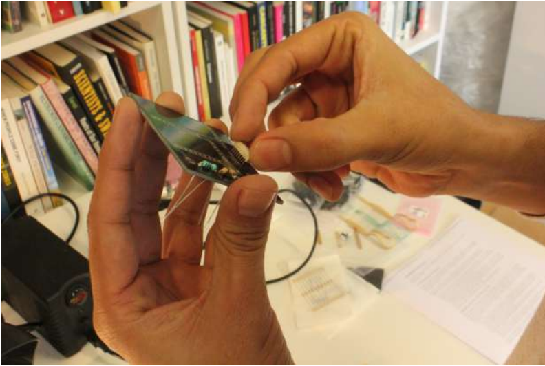
Insert the Molex PicoBlade connector in to the PCB slot
