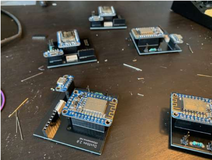
Dustboxes with breakout boards attached
