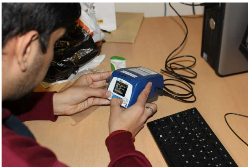
Configuring the Sidepak for calibration
